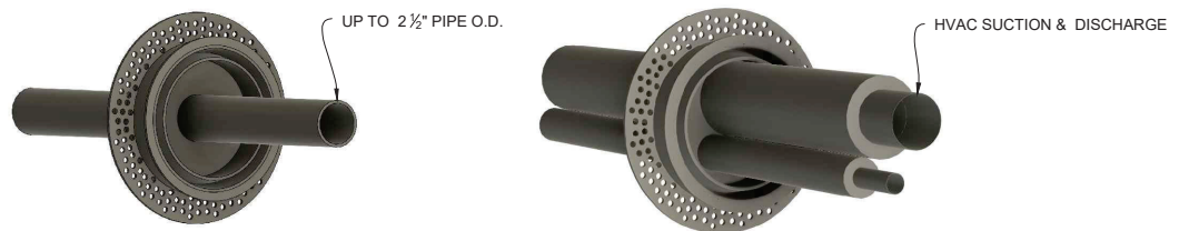
PIPE EXPANSION RING INSTALLATION DETAIL
